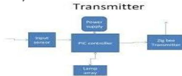
Fig.1 Zigbee Transmitter block diagram
