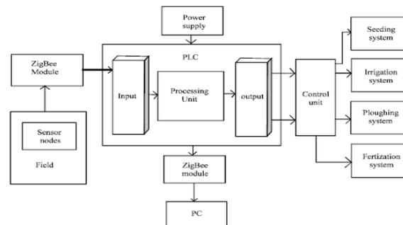
Fig. 3 Block Diagram representing ZigBee processing
