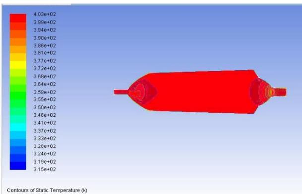
Fig. 7 (a) Static Temperature results of Existing model
