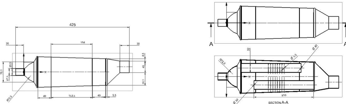
Fig. 1 Two Dimensional model of Existing Silencer (Top View) and 2D model of existing silencer (Front and Sectional view)
