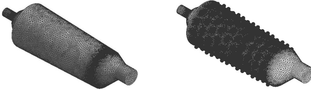
Fig. 6 Meshed model of existing and modified staggered model
