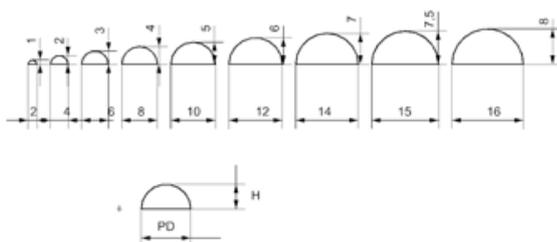
Fig. 2 (a) Dimension of Dimples
