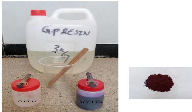
Fig. 1 Polyester resin and haematite ( $Fe_2O_3$  particles)
