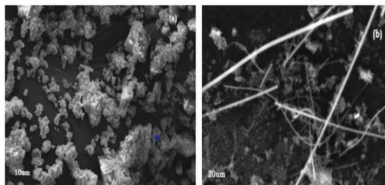
Fig.4 (a) SEM image of Ni<sub>30</sub>/ZnO catalyst before and (b) SEM image of Ni<sub>30</sub>/ZnO catalyst after hydrogen production reaction.
