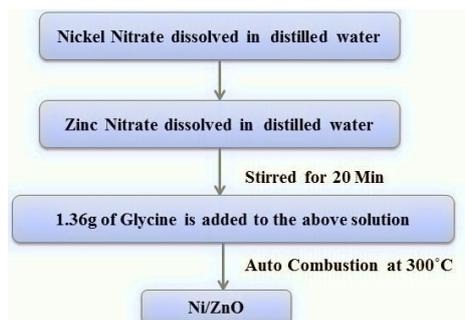
Flow chart-1 Synthesis of Nickel supported Zinc Oxide catalyst
