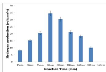
Fig.1 Effect of reaction time on hydrogen production (Volume %) with Ni30/ZnO catalyst
