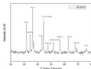
Fig.3 XRD plot of Ni30/ZnO catalyst after hydrogen production reaction
