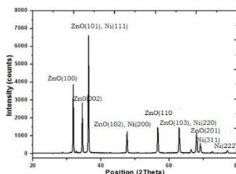
Fig.2 XRD plot of Ni30/ZnO catalyst before hydrogen production reaction
