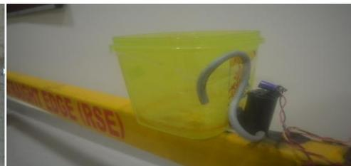
Fig. 6 Water Dispenser (with Dye Marker)
