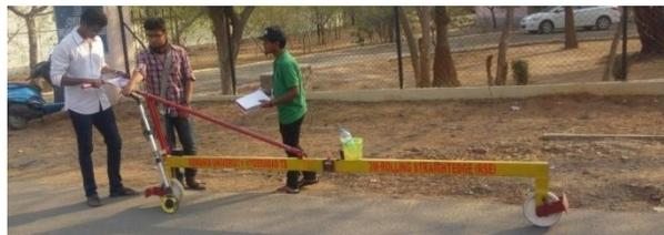
Fig. 7 Photos depicting during measurement of Smoothness of Roads in Osmania University by Using ERSE
