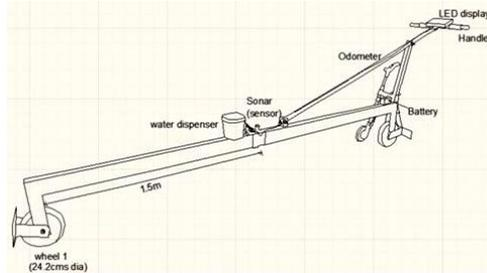
Fig. 1 Component Details of Electronic Rolling Straight Edge (ERSE)
