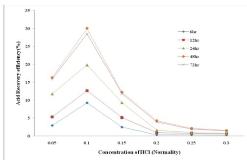
Fig.3 Acid recovery efficiency obtained at different time intervals and concentrations.
