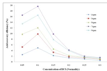
Fig. 2 Acid recovery efficiency of synthetic solutions at different flowrates and concentrations
