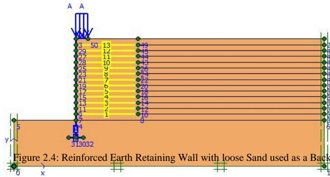
Figure 2.4: Reinforced Earth Retaining Wall with loose Sand used as a Backfill Material.
