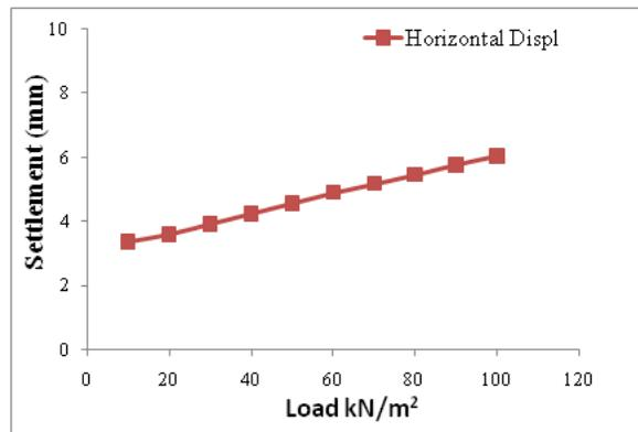
Figure 3.5: Load Displacement Relationship for Dense Sand (Horizontal Displacement).
