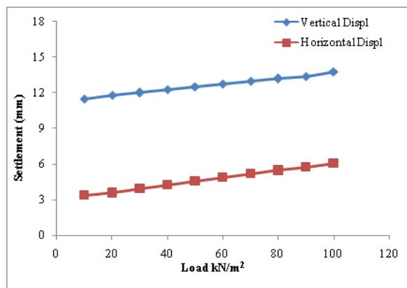
Figure 3.6: Comparison of Load Displacement Relationship for Dense Sand.
