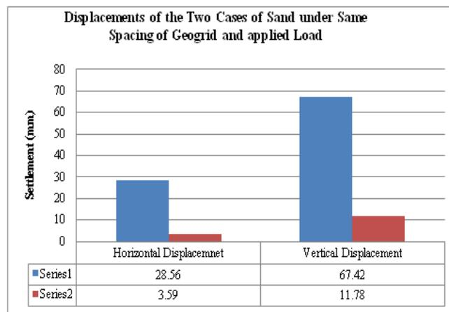
Figure 3.7: Displacements of the Two Cases of Sand under Same Spacing of Geogrids and applied Load.
