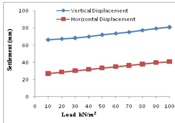
Figure 3.3: Comparison of Load Displacement Relationship for Loose Sand
