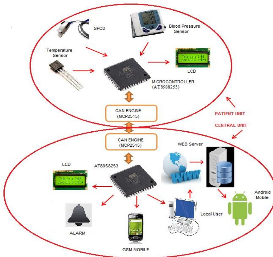
Fig. 1 Architectural Block diagram of smart & secure multi patient monitoring system)
