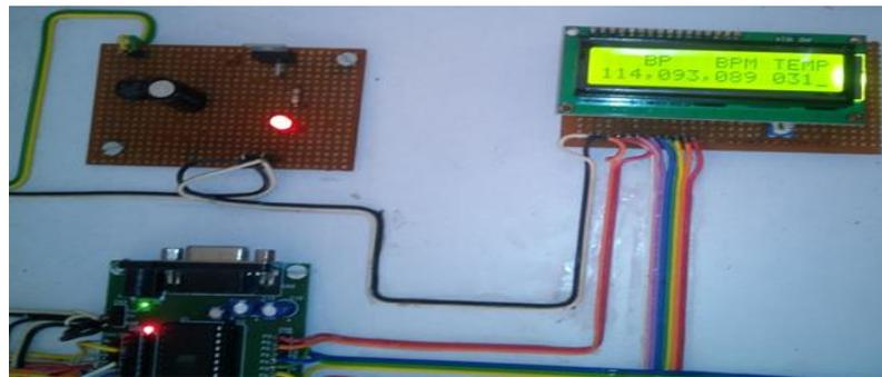
Fig. 3 Data transmitted to the LCD
