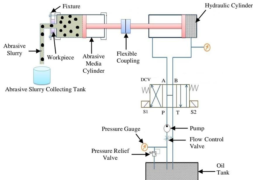
Fig. 1 Schematic diagram of abrasive flow machine
