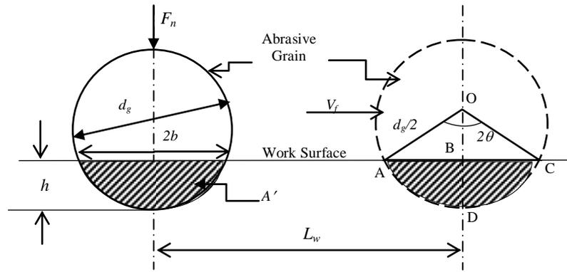
Fig. 2 Schematic diagram of a spherical abrasive grain
