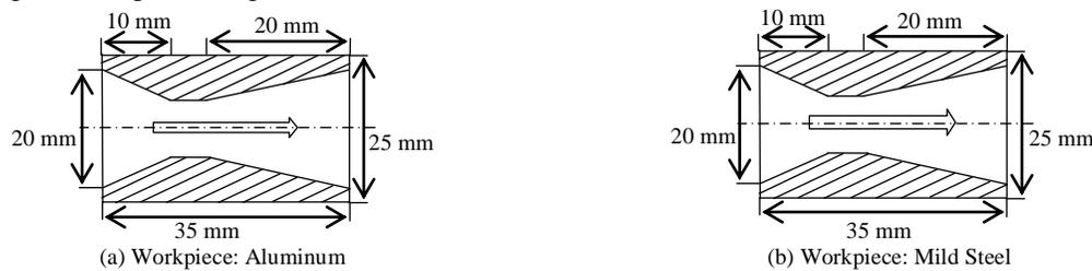
Fig. 3 Convergent-Divergent Workpiece
