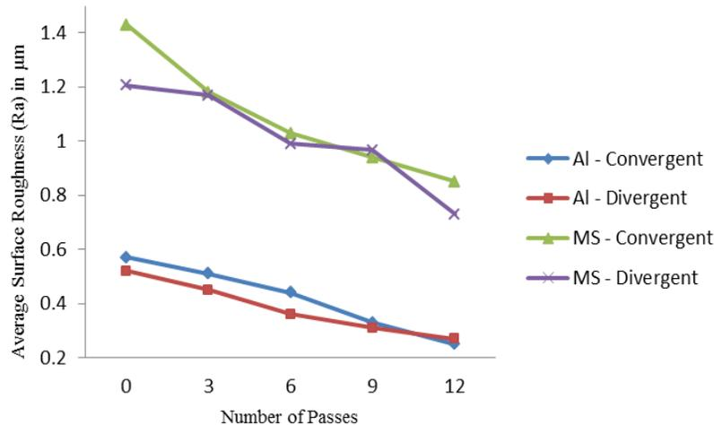
Fig. 4 Number of Passes Vs Average Surface Roughness
