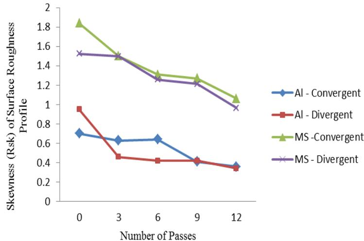
Fig. 5 Number of Passes vs Skewness of Roughness Profile
