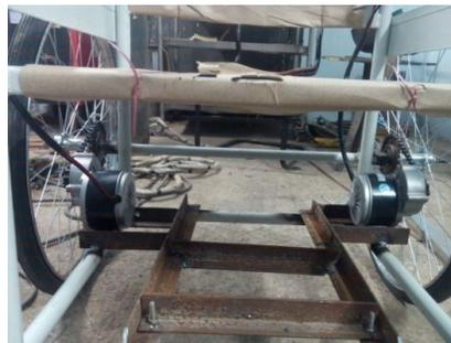
**Fig 6.1 Wheel chair Motors Alignment**
