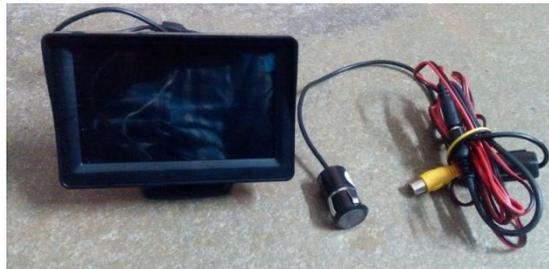
**Fig 5 Rear View Camera and Display**
