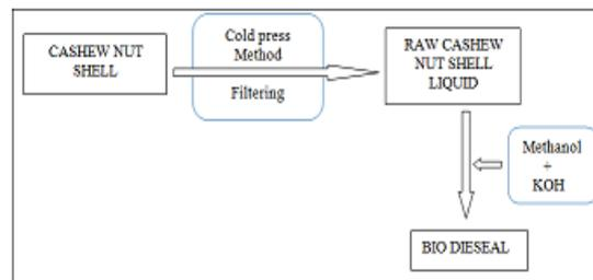
Fig. 1 Extraction of CNSO and Transesterification Process
